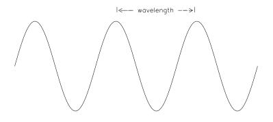
Figure 1: *Wavelength* is the distance between wave peaks.
