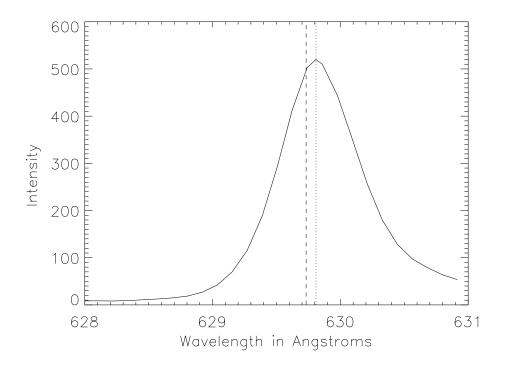
Figure 6: Emission line profile for an oxygen atom that has lost four electrons. The peak intensity is shown by the dotted vertical line, and occurs at 629.809 Å. The rest wavelength of the line, 629.732 Å, is shown by the dashed vertical line.
