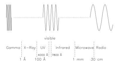
Figure 2: The *electromagnetic spectrum* contains light waves of all different wavelengths. The symbol "Å" means "Angstrom", a unit of length often used to describe wavelengths of light. One Angstrom is one ten-billionth, or  $10^{-10}$ , of a meter. Notice that the fraction of the electromagnetic spectrum that is visible to the human eye is fairly small.
